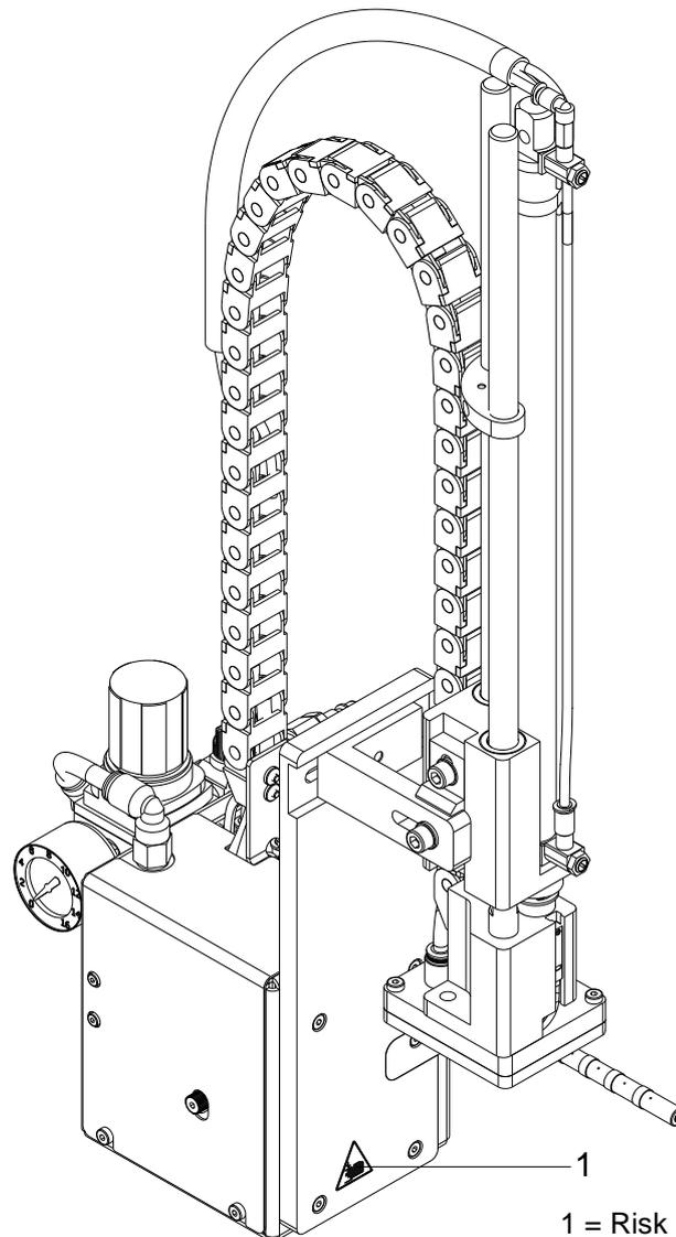
1 = Risk of crushing due to the movement of the pad
