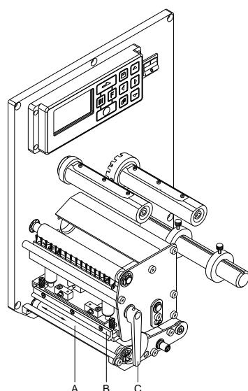
A soiled print roll can lead to reduced print quality and can affect transport of material.
