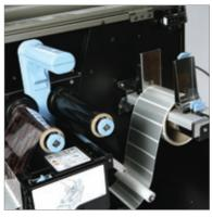
Colour-coded mechanisms for faster user training time
