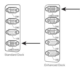
The CANbus/Audio connector is a D-15 male connector located on the back of the dock.
