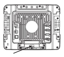
It may be desirable to secure the Thor VM2 in the dock so it cannot be removed from the dock. The quick release handle on the Thor VM2 is notched to allow a user supplied standard padlock to be placed through a hole in the bracket on the back of the Thor VM2 in the location shown below. Once the padlock is installed, the release handle cannot be moved so the Thor VM2 cannot be removed from the dock. The padlock shackle must be smaller than 3/16" (4.76mm).
