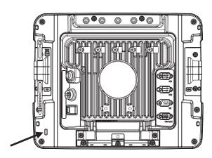
The Thor VM2 can be secured with a standard laptop security cable using the slot on the back of the Thor VM2.
