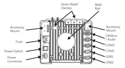
**Note:** For the VMX Enhanced Dock: COM1 is used for screen blanking (via the power cable connector) and is unavailable when the screen blanking box is attached. When a screen blanking box is attached, any external serial device such as a scanner, must be connected to the COM2 port on the dock. If a screen blanking box is not connected via the power cable, the COM1 port on the dock is available for a serial device
