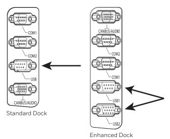
The USB or USB1 connector is a D-9 female connector located on the back of the dock. See USB and USB1 Connector for connector pinout detail.
