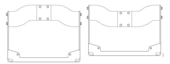
Additionally, the slotted U bracket allows the Thor VM2 to be mounted vertically or tilted forward or backward for best viewing angle.
