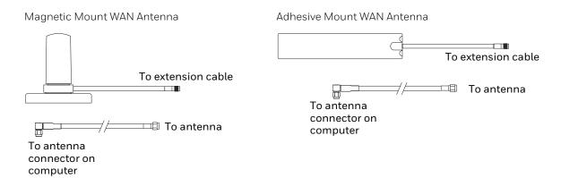
The Remote Antenna Installation Kit consists of the WAN antenna and an extension cable. The remote antenna is mounted on the top of a forklift, truck or other vehicle and cabled to the Thor VM2 inside the vehicle.
