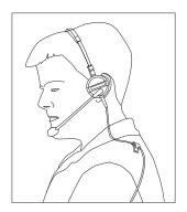
The headset consists of an earpiece, a microphone, a clothing clip and a cable.
