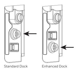
Power is supplied to the Thor VM2 through the power connector. Additionally this assembly provides a connection point for the vehicle's chassis ground to be connected internally to the conductive chassis of the computer.
