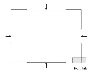
The protective film is slightly larger than the Thor VM2 touch screen, however the notches on the edge of the protective film (indicated by the arrows) correspond to the display size of the Thor VM2. The protective film is not adhesive. The corner edges are designed to fit between the Thor VM2 display and the display housing to hold the protective film in place.
