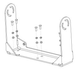
After the bottom bracket has been attached to a rigid surface, you are ready to assemble the Thor VM2 bracket configuration.
