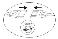
3. Slide the cable ends together until they click shut. Do not twist or bend the connectors. The Thor VM2 internal microphone and speakers are automatically disabled when the headset is connected.
