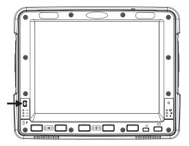
Press the power button to turn the Thor VM2 on. When the Windows desktop is displayed or an application begins, the power up sequence is complete.
