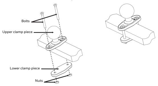
Position the upper clamp piece with ball on the beam. Place the bolts through the holes in the upper clamp piece.
