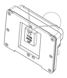
The dock contains a tethered I/O Pin Cover to protect the I/O pins on the dock when a Thor VM2 is not mounted in the dock.
