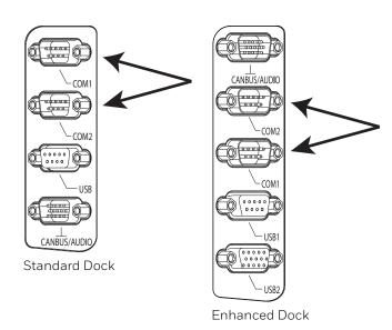
The COM1 and COM2 connectors are D-9 male connectors located on the back of the dock.
