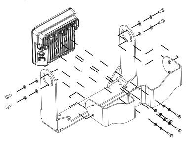
Note: For the steps below, always place the lock washer on the bolt before the flat washer.
