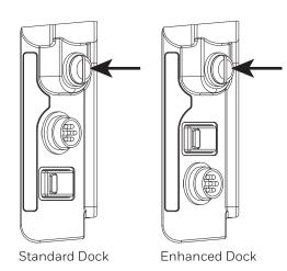
The Thor VM2 uses an 8A time delay (slow blow) fuse that is externally accessible and user replaceable. The fuse is located on the back of the dock. The fuse is accessed by unscrewing the cap as indicated.
