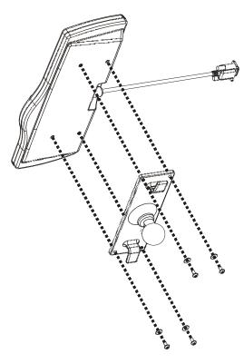
**Note:** Excess keyboard cable length can be looped around the hooks on the bottom of the keyboard mounting plate.
