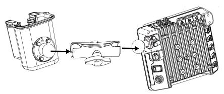
5. Tighten the knob on the RAM arm while adjusting to the desired angle.
