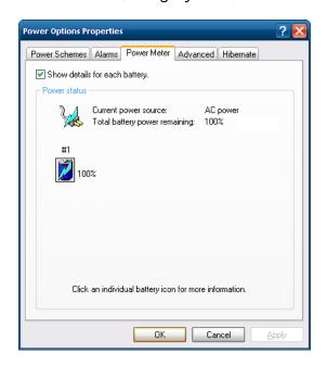
On the **Power Meter** tab, battery #1 refers to the UPS battery.
