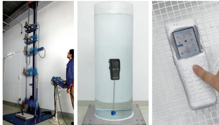
3-meter drop resistance test
